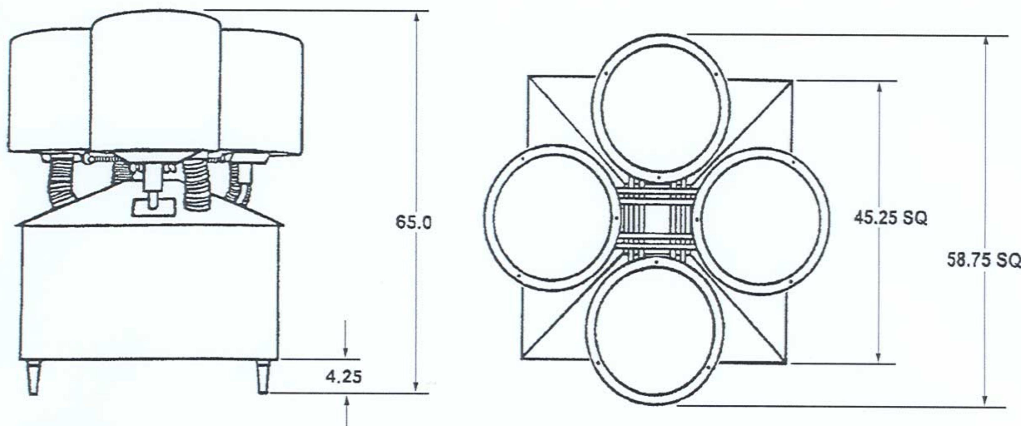
Rotation Pattern: Each beam moves in a conical motion around an axis tilted 22.5 degrees from the vertical. Solid angle of the cone is 45 degrees. Four beams synchronized, creating a cloverleaf pattern.
