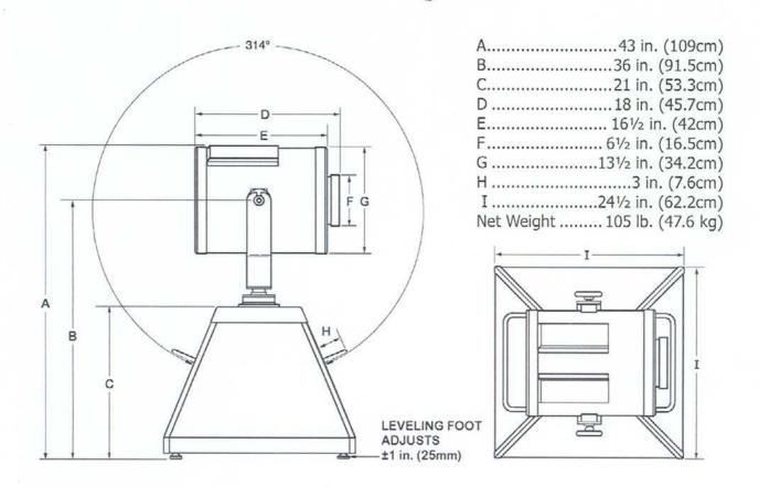
Power Requirement: 110-120 V.AC, 15 Ampere Single Phase (220-240 volt model available) Bulb: Single-Ended 1200 Watt Metal Halide (Philips MSR/MSD 1200/2 or equivalent)
